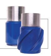
These are the newest couplings in the Tuff-Kote Line-Up and are designed with well optimization in mind. By creating shorter and spiraled designs, we have decreased the restriction at each sucker rod joint. This in turn decreases the pressure drop across the coupling allowing for optimal production from the well.
